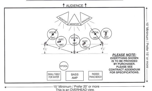
Please note the close-in semi-circle setup with outside mics angled 30° from axis and arc set about 11/2′ ahead of center mic. Vocal mic heads should be about 3′ apart. Monitor speakers should be touching each other. Please use round-based mic stands - NOT TRIPODS - particularly on the stands for the instrument mics. Please **do not** wrap the mic cords around the stands!
